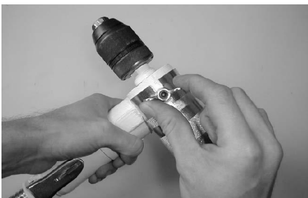
5. Secure safety guard with wing nuts.
