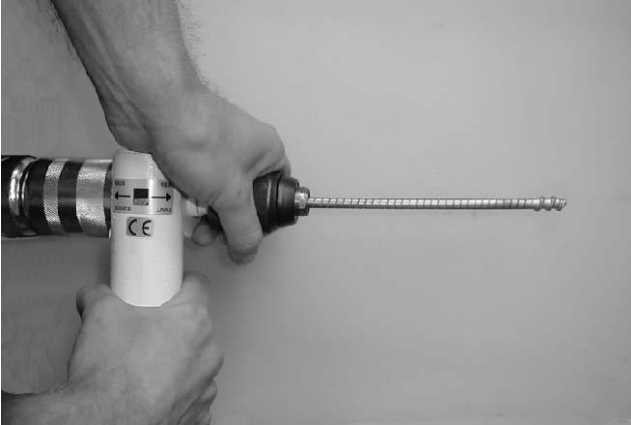
9. Clamp the pin approx. 30cm from the screw end in the quick clamp chuck for the optimum working length.
