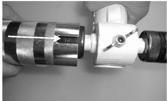
4. Slide safety guard on quick clamp chuck on the opposite of working side.
